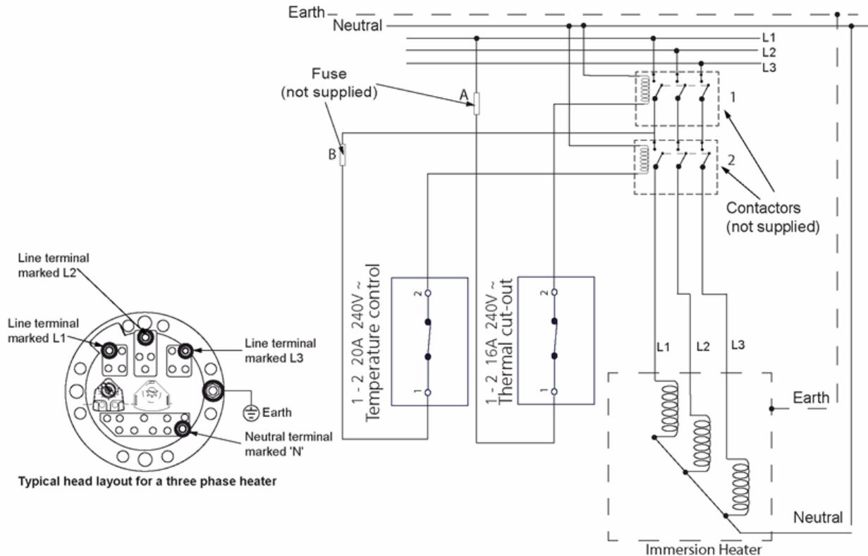
FIGURE 6: 3 phase wiring schematic
