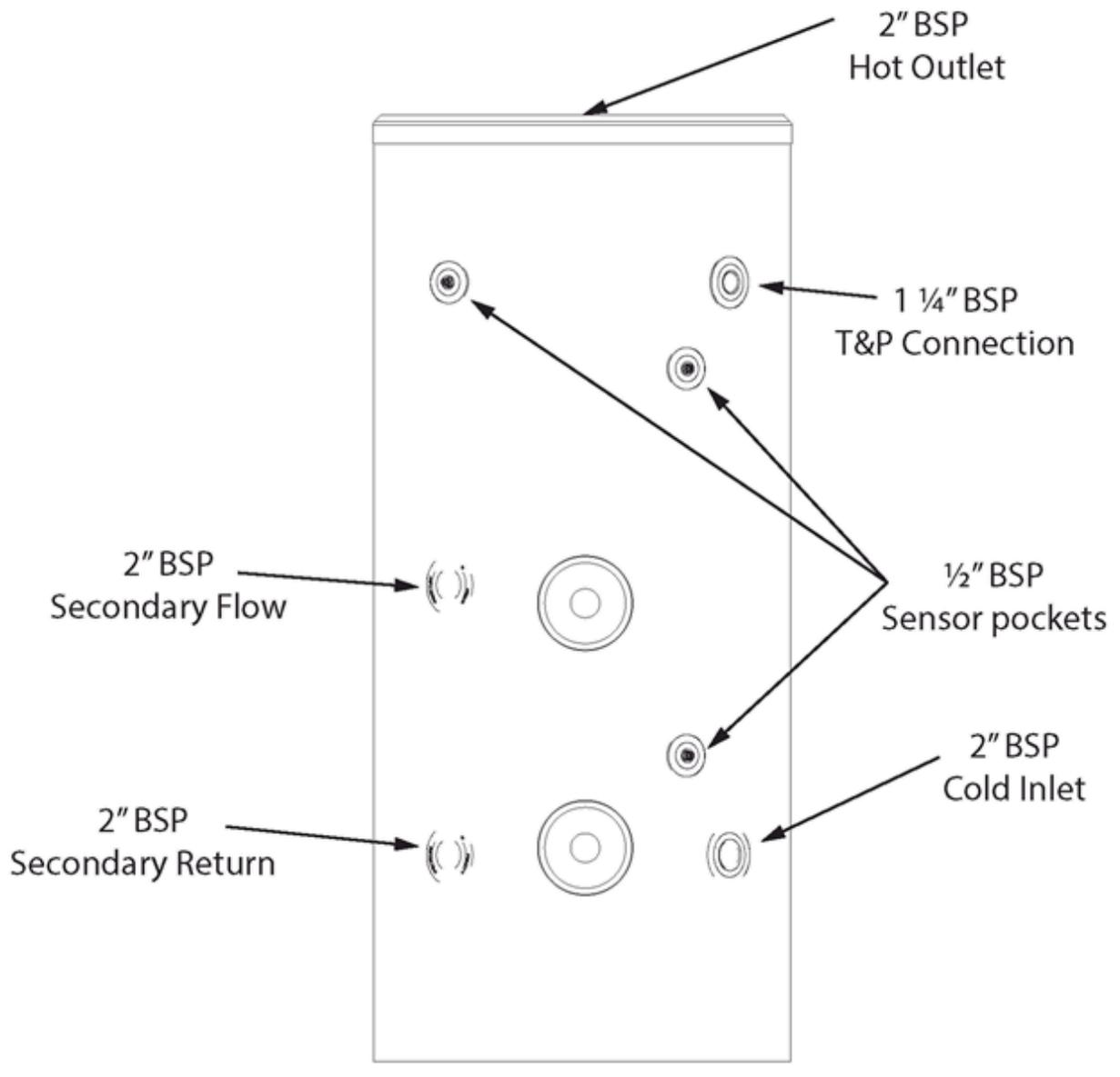
FIGURE 3: Flexistor Connections
