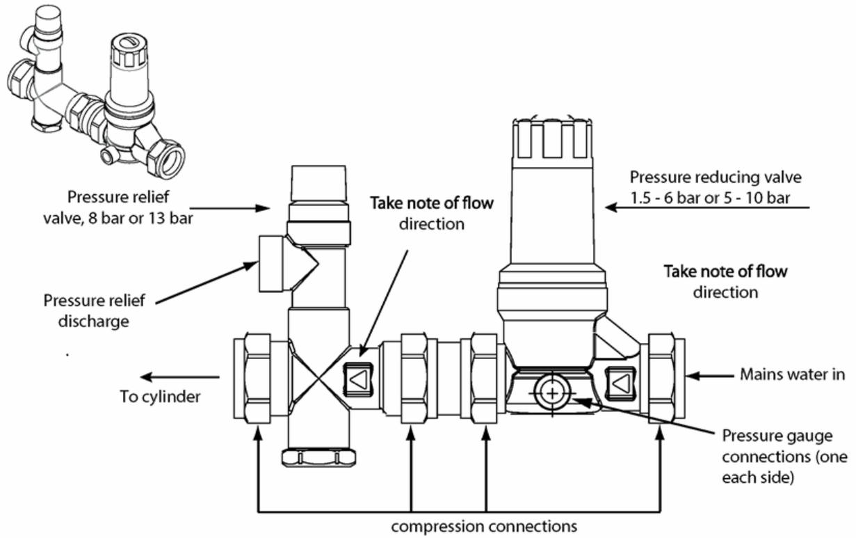
Figure 07: Cold water combination valve (for 400 & 500ltr)
