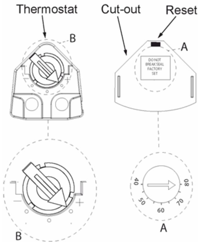
FIGURE 4: Thermostat and thermal cut-out settings
