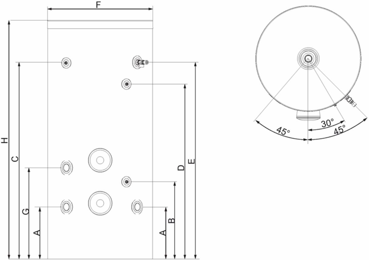
FIGURE 2: Flexistor Dimensions
