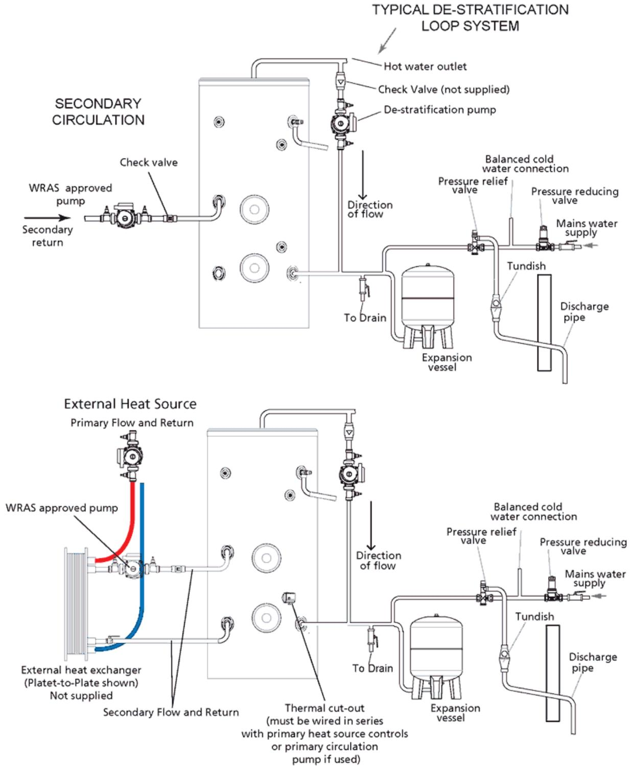
Figure 09: Schematic installations
