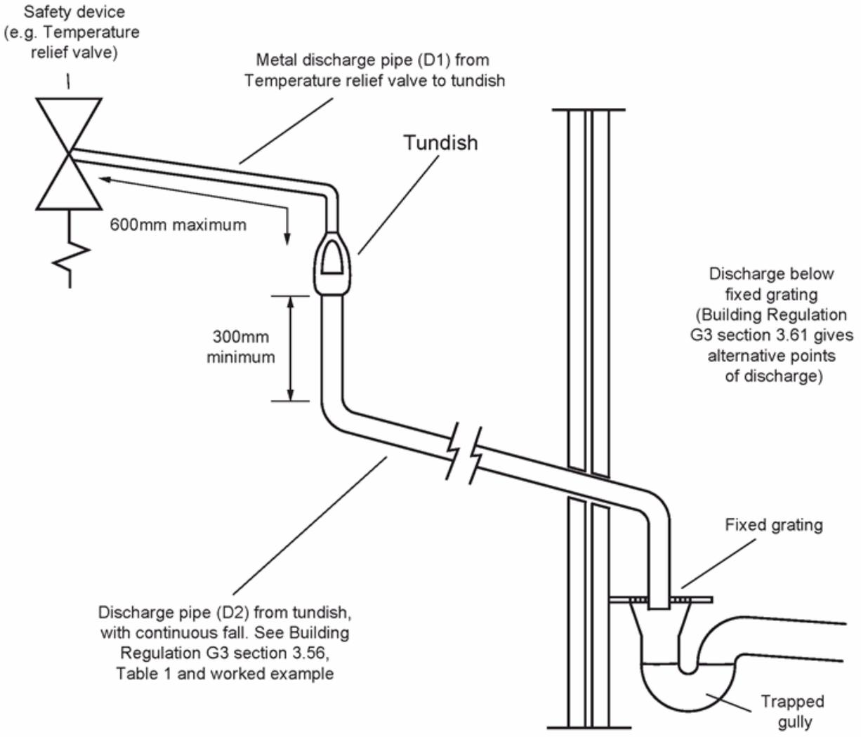
Figure 10: Typical discharge pipe arrangement (Extract from Building Regulations G3 Guidance section 3.5 to 3.63)
