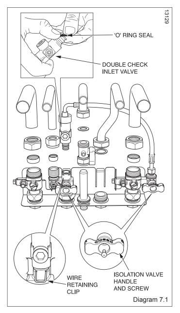
Fit the Central Heating Isolation Valve handles and secure with screws provided.
