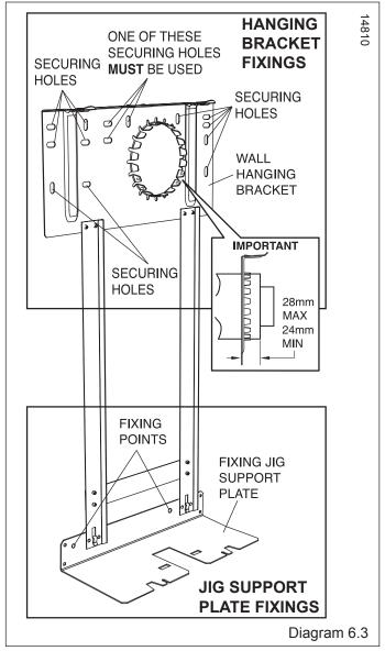
**Direct Rear Flue only** - The flue can now be pulled back through the hanging bracket and secured as shown in diagram 6.3.
