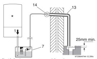
Fig. 13 Condensate pump to external disposal
