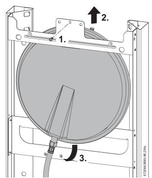
Fig. 137 Removing expansion vessel from wall frame
