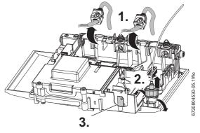
Fig. 117 Replacing the controls (SMPS)
