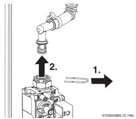
Fig. 86 Gas valve connection
