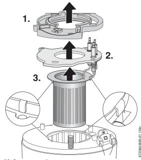
Fig. 89 Burner removal
