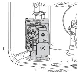
Fig. 67 Inlet pressure test point
