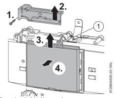
Fig. 52 Removing the blanking panel
