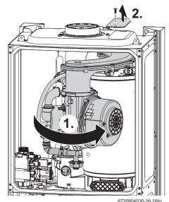
Fig. 88 Rotate air/gas manifold
