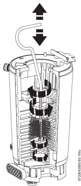
Fig. 92 Cleaning heat exchanger
