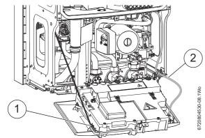
Fig. 120 Support cable connection
