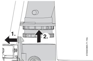
Fig. 110 Release lower exhaust connection
