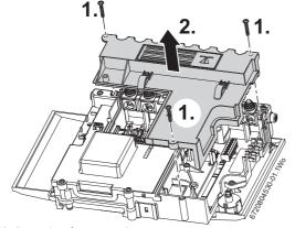
Fig. 50 Removing the connection cover
