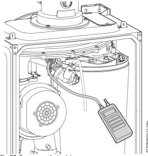
Fig. 80 Fan pressure test point
