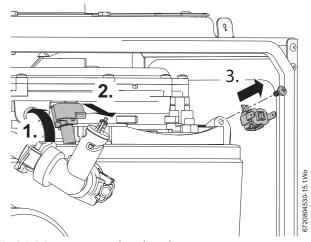
Fig. 94 Primary sensor and overheat thermostat
