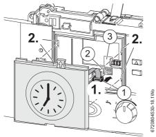
Fig. 53 Plug in connector
