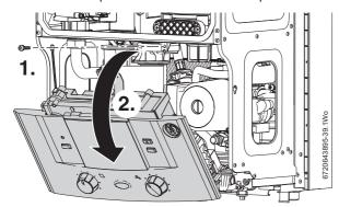
Fig. 49 Moving control panel into the service position
