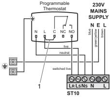
Fig. 59 Programmable thermostat
