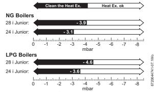
Fig. 81 Fan pressure readings
