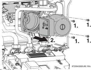
Fig. 126 Pump head removal
