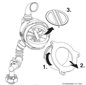
Fig. 103 Flap valve assembly
