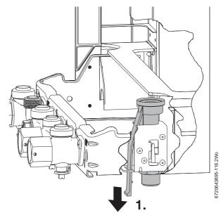
Fig. 30 PRV connection in the down position
