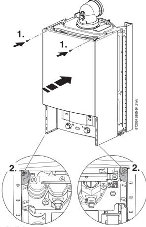
Fig. 71 Fitting case
