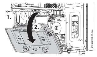
Fig. 97 Control panel to service position
