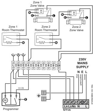
Fig. 55 Two room thermostats, one external timer
