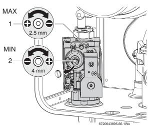
Fig. 85 Gas valve adjustment
