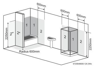
Fig. 17 Bathroom installations
