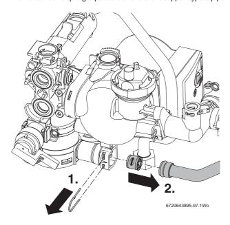
Fig. 135 Removing the bypass valve
