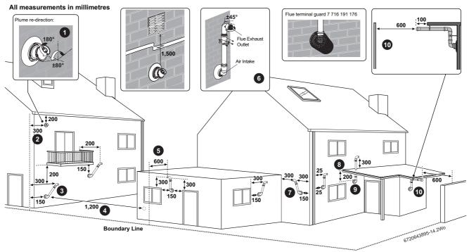
Fig. 21 Plume terminal positions
