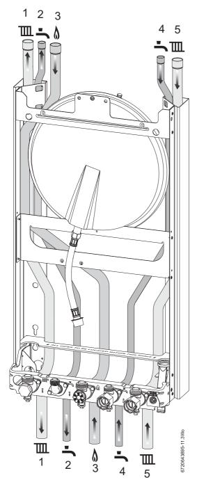
Fig. 19 Plumbing manifold
