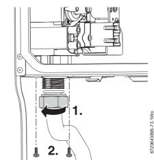
Fig. 99 Gas valve lower connection
