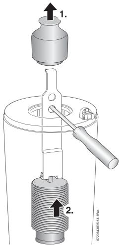
Fig. 90 Baffle removal
