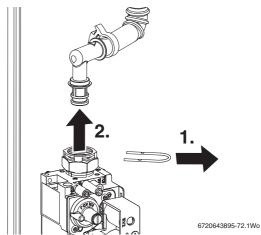
Fig. 98 Gas valve upper connection
