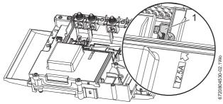
Fig. 114 Fuse location (SMPS)
