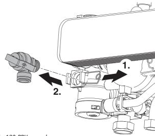
Fig. 132 PRV removal
