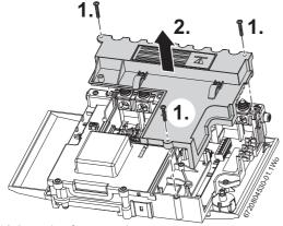
Fig. 113 Removing the connection cover
