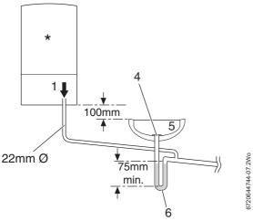
Fig. 9 Disposal to a waste pipe
