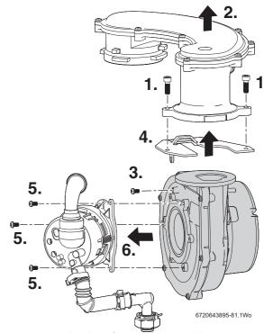
Fig. 102 Dismantling the air/gas manifold assembly
