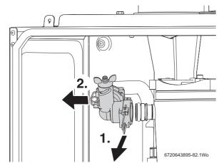
Fig. 108 Flow pipe removal
