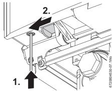
Fig. 119 Control unit release
