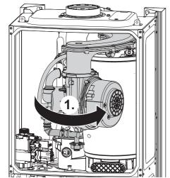
Fig. 101 Rotate the air/gas manifold assembly
