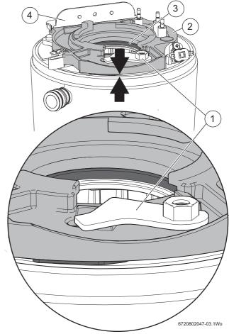
Fig. 105 Initial location of the clamping plate
