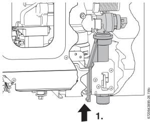
Fig. 32 PRV in the up position
