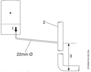
Fig. 8 Disposal to soil vent stack
