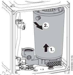
Fig. 112 Heat exchanger removal
