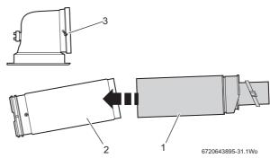
Fig. 37 Reducing the standard terminal
