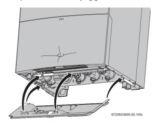
Fig. 72 Bottom panel installation
