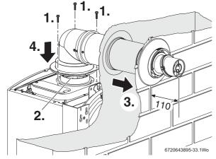
Fig. 41 Telescopic flue installation
