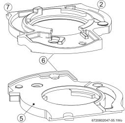
Fig. 106 Clamping plate detail
