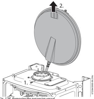
Fig. 136 Removing the expansion vessel
