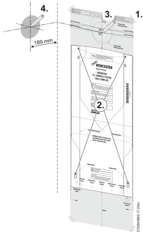
Fig. 23 Marking the flue position
