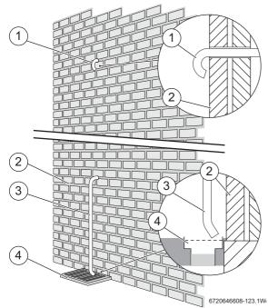
Fig. 15 Pressure relief pipe work
