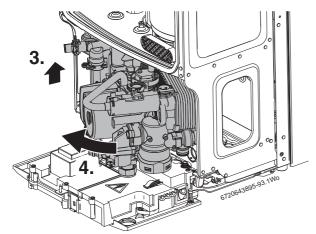
Fig. 131 Hydraulic block removal part 2
