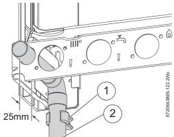
Fig. 28 Condensate drain pipe work detail
