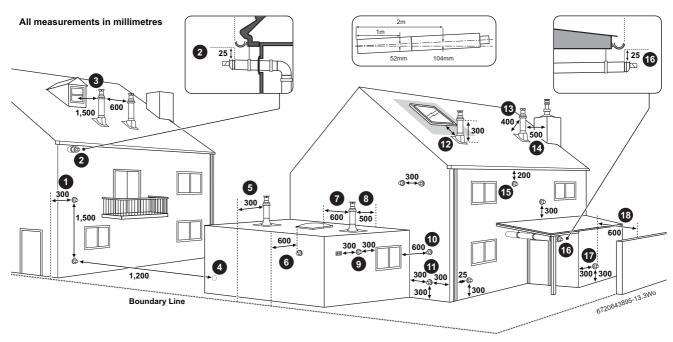
Fig. 20 Flue terminal positions
