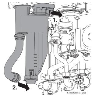
Fig. 47 Fitting syphon
