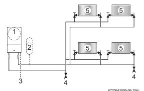
Fig. 6 Existing build - Sealed system
