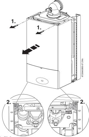
Fig. 73 Remove outer case
