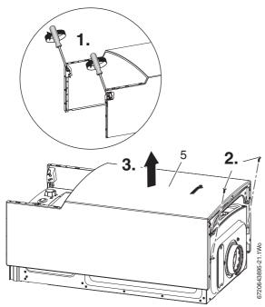
Fig. 27 Outer case screw removal
