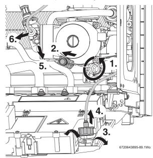
Fig. 129 Drain tap and pressure gauge removal
