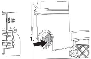
Fig. 96 Remove thermostat
