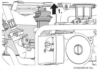
Fig. 124 Auto air vent removal
