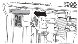
Fig. 45 Remove blanking cap
