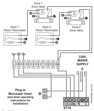
Fig. 56 Two room thermostats, one integrated timer
