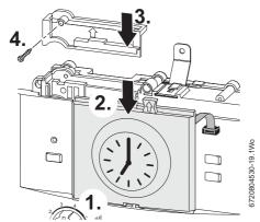
Fig. 54 Securing the module into the control panel
