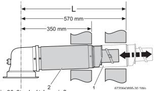
Fig. 36 Standard telescopic flue
