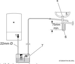
Fig. 10 Condensate pump disposal
