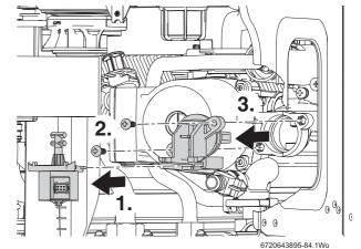
Fig. 122 Diverter valve and motor
