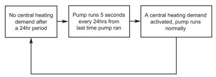
Fig. 140 Protection functions
