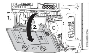
Fig. 74 Control panel into service position
