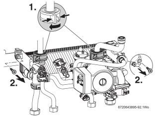
Fig. 130 Hydraulic block removal part 1
