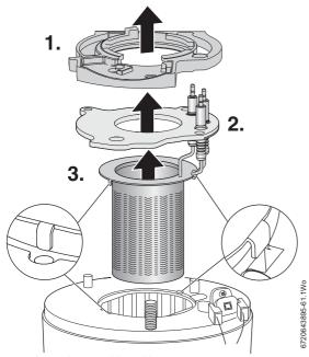
Fig. 104 Electrode assembly and burner
