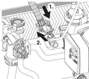
Fig. 34 Expansion vessel hose connection
