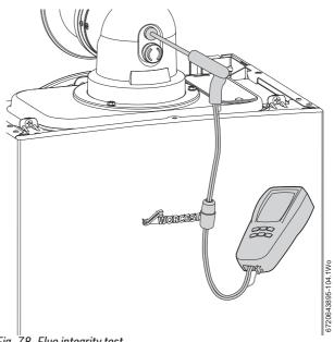
Fig. 78 Flue integrity test
