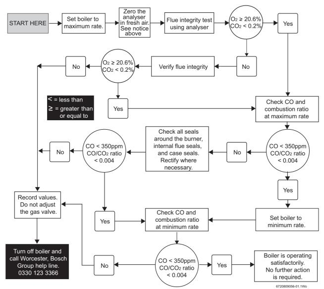
Fig. 70 Combustion check flow chart
